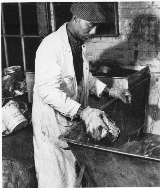
At a grease refinery the first steps in converting household fats and greases to glycerin include heating the fats and pouring them into "buggies" to be wheeled into the refining room. OWI Photo
